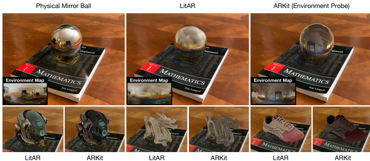
Fig. 1. Rendered objects with LitAR compared to a physical mirror ball and with ARKit [34]. Row 1: LitAR produces visually-coherent reflective rendering while ARKit fails; the bottom part of the ARKit-rendered ball does not faithfully reflect the book cover. The top part of the LitAR-rendered ball has an intentionally gradient blurring effect for quality-performance trade-offs (see §4.2). Row 2: LitAR achieves more realistic and visually coherent rendering effects than ARKit for objects with different materials.
