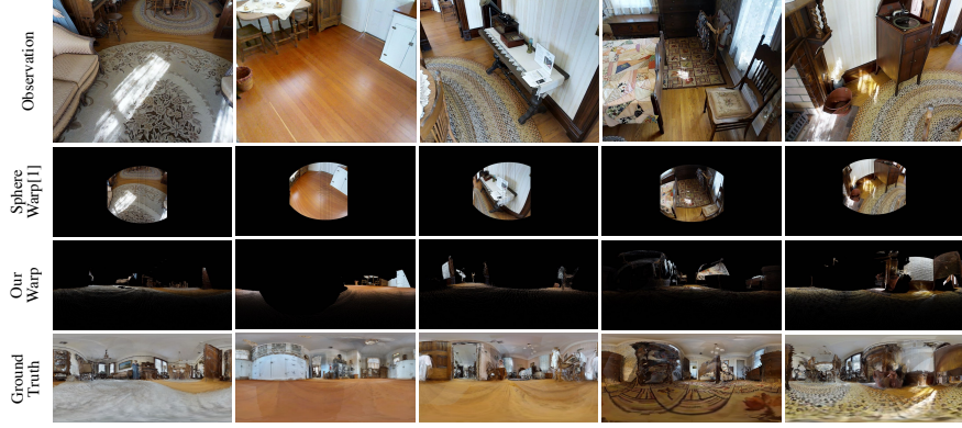
Fig. 3. Comparison of different warping methods. To transform mobile camera view spatially, i.e., from observation to rendering location, we leverage the point cloud which was generated from the RGB-D image. Our approach does not subject to distortion problem and therefore is more accurate than spherical warping that only considers RGB image [13].
