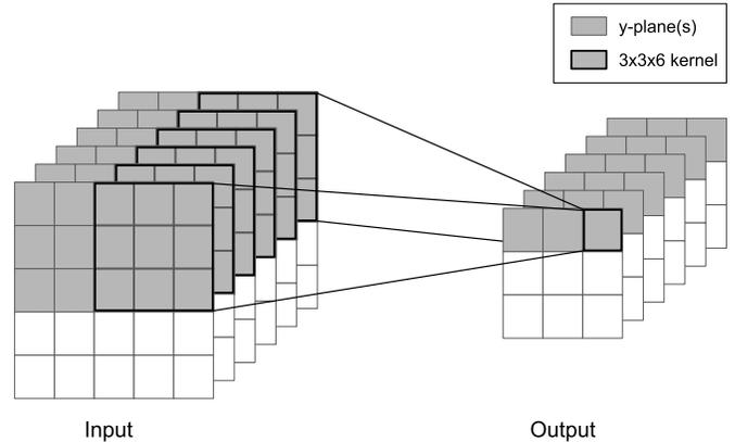
**Fig. 1: Illustration of Y-Plane Partitioning.** A 5x5x6 input is convolved with a 3x3x6 kernel. This figure highlights the computation of 1 output value. Three input y-planes are required to compute one output y-plane.
