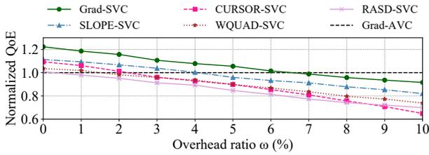
**Figure 5: Impact of coding overhead.** QoEs were obtained with  $\omega$  increasing from 1% to 10% in simulation, normalized to Grad-AVC.
